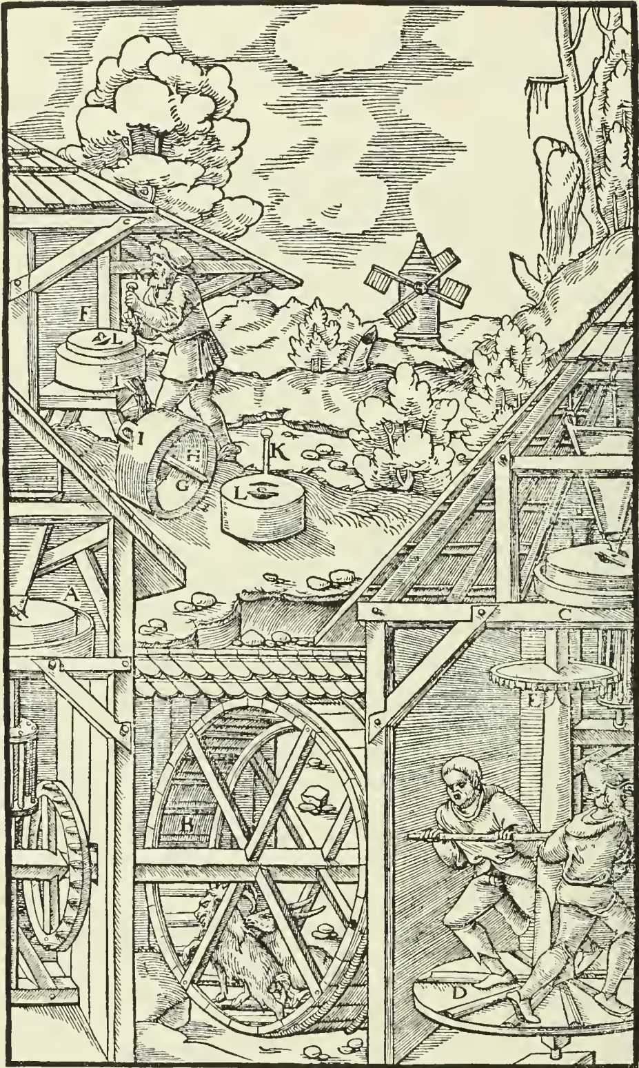
A—FIRST MILL. B—WHEEL TURNED BY GOATS. C—SECOND MILL. D—DISC OF UPRIGHT AXLE. E—ITS TOOTHED DRUM. F—THIRD MILL. G—SHAPE OF LOWER MILLSTONE. H—SMALL UPRIGHT AXLE OF THE SAME. I—ITS OPENING. K—LEVER OF THE UPPER MILLSTONE. L—ITS OPENING.
